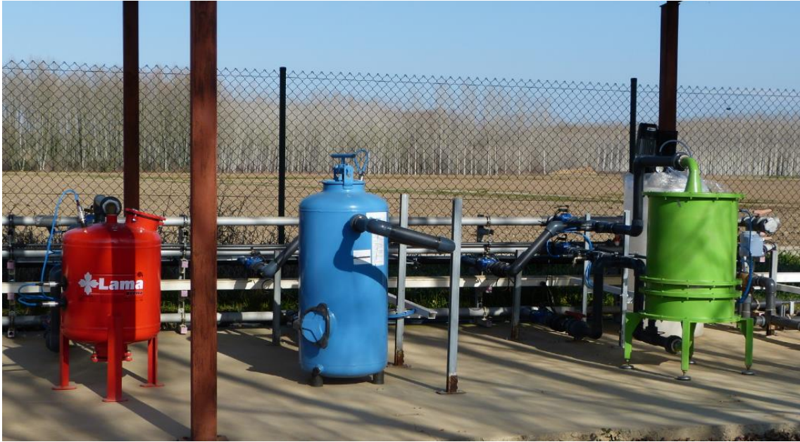
Fig. 1 - Picture of the experimental set-up with the three filter designs: (a) red: arm collector; (b) blue: inserted domes; and (c) green: porous media prototype.
