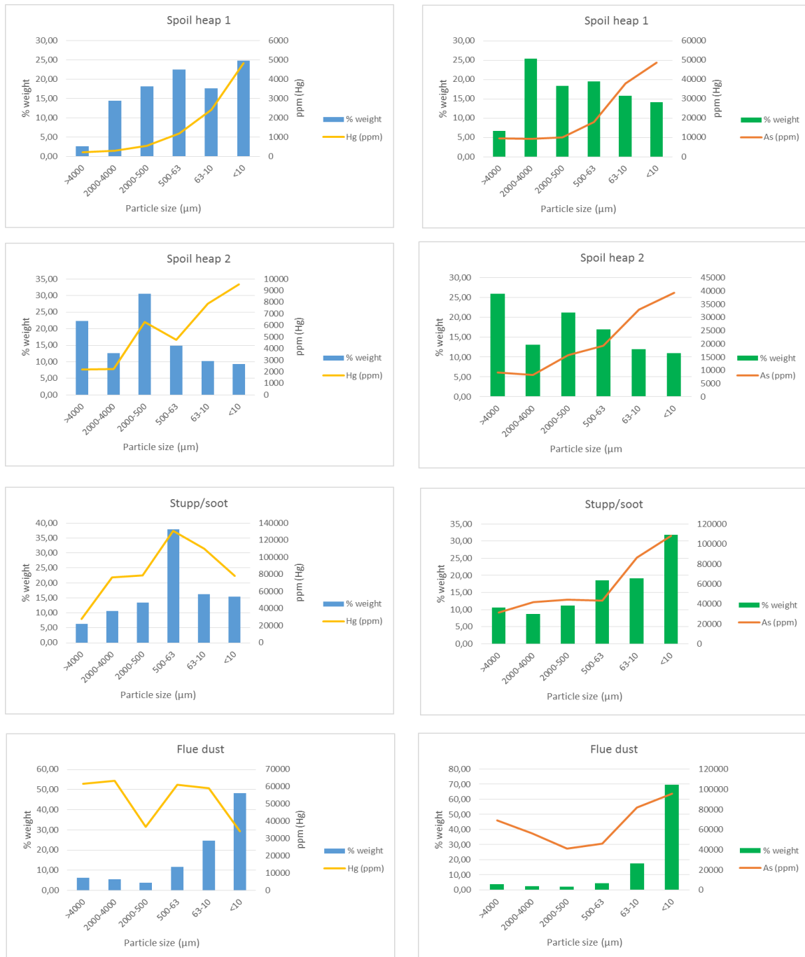
368 Figure 4: Distribution of Hg (left graphs) and As (right) in the representative 369 subsamples of mining and metallurgical waste subjected to grain-size fractionation by 370 wet sieving, and subsequent ICP-MS determination of elemental contents.
