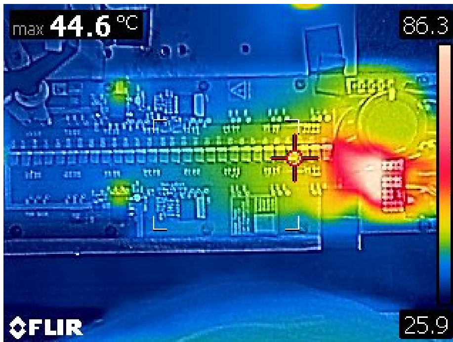
Figure 6-32: Thermal image of the PCB
