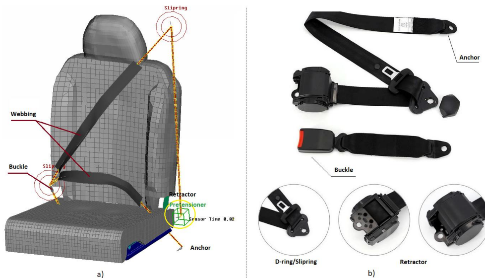
Figure 1.3: a) Initial 3-point seat belt model with slirings, a retractor and a pretensioner and b) illustration of real belt components, image adapted with permission from [13].
