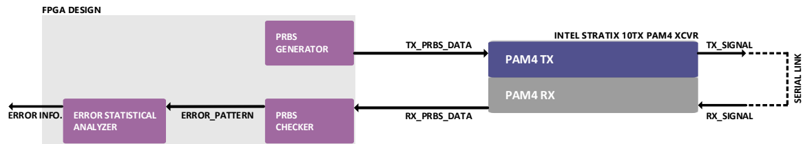
Figure 1.1.- PAM4 signal integrity analysis system simplified schema including main design units involved in signal generation and processing (note that this schema is a reduced version of the system diagram shown in figure 5.1).
