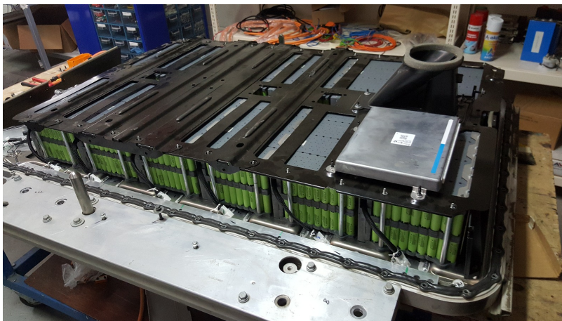
Figure 1-18: Renault Zoe battery pack
