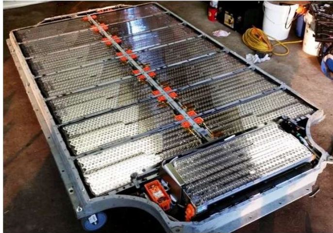
Figure 1-16: Tesla model S 85kWh battery pack
