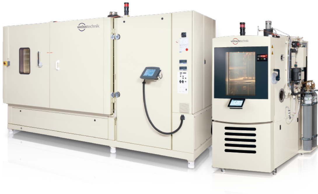
Figure 3-6: Weiss technik climatic chamber
