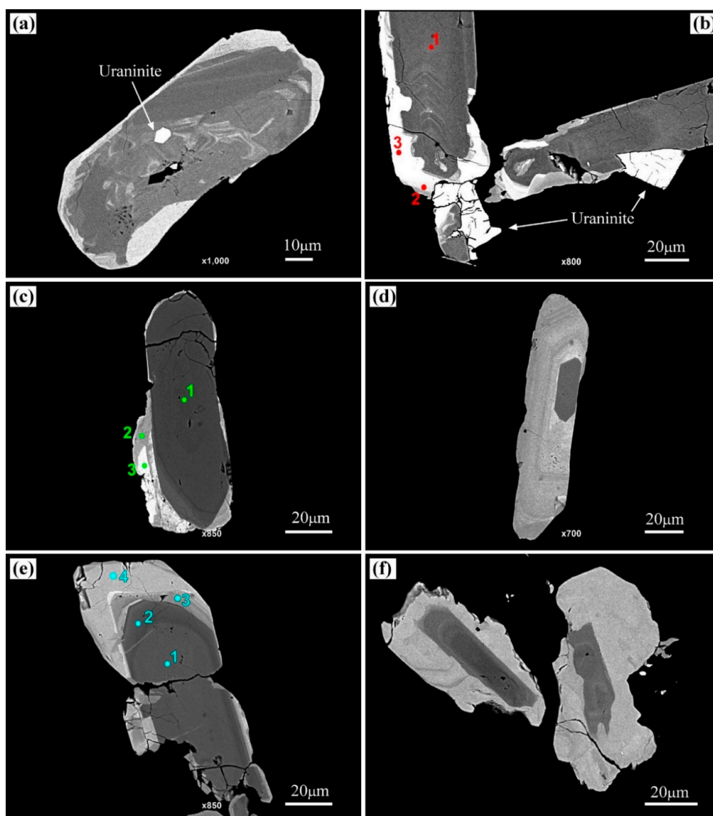
Figure 8. SEM-BSE images of columbite–tantalite crystals from the Presqueira pegmatite. In these images, the darker the grey color is, the richer is the composition in Nb. Numbers and dots (red, green, and blue) correspond to the zone of the crystal plotted in the compositional columbite–tantalite quadrilateral of Figure 10; (a) euhedral prismatic crystal of columbite–tantalite with an inclusion of a tiny uraninite crystal. The columbite–tantalite grain shows a discontinuous oscillatory-zoned core, with mainly columbite-(Fe) composition partially corroded by Nb-poorer patch with complex zoning, surrounded by an irregular thinner rim with embayments of tantalite-(Fe) composition; (b) columbite–tantalite grains with tiny uraninite crystals attached at their borders. Note the left-hand crystal showing a fine-oscillatory zoned core, columbite-(Fe), a Nb-poorer irregular rim with complex zoning, and a lobulated rim of tantalite-(Fe) composition; (c) a prismatic columbite–tantalite crystal with oscillatory zoning in the core, columbite-(Fe), a Nb-poorer irregular rim with complex zoning, and a narrow rim of mostly tantalite-(Fe) composition; (d) a prismatic columbite–tantalite crystal showing a small homogenous core of columbite-(Fe) and a thicker fine-oscillatory zoned rim of chiefly tantalite-(Fe) composition; (e) euhedral oscillatory zoned columbite–tantalite grain exhibiting truncated layers suggesting episodes of partial dissolution and successive crystallization; (f) sub-euhedral columbite–tantalite grains showing fine-oscillatory zoned cores, mostly columbite-(Fe), and thick fine-oscillatory zoned rims of mainly tantalite-(Fe). In the right-hand crystal, note the core containing inward-penetrating embayments of the rim. In the right-hand of the image, the bright tiny crystals are uraninite.
