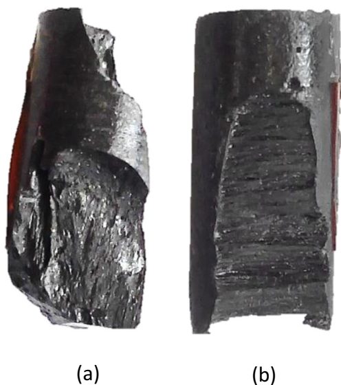
Fig. 7. Images of the polyester composites: a) longitudinal and b) transverse configuration.
