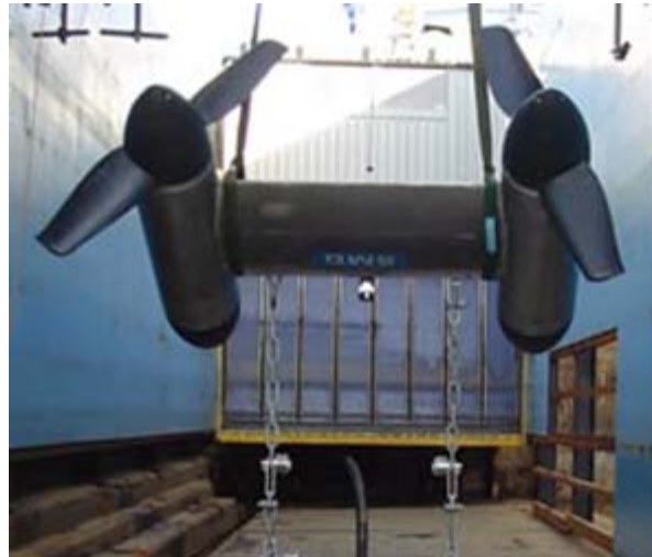
Fig.33 Turbina TidEL, SMD Hydrovision (REUK, 2018b)
