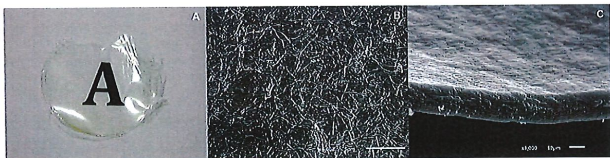
Fig 3. (A) Macro photograph appearance of HPCM, (B) SEM microphotograph displaying fibrillary ultrastructure and (C) thickness of HPCM.
