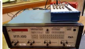
(e) Constant temperature anemometer and Data acquisition system
