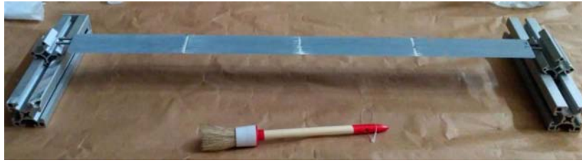
Figure 5.10: Manufactured blade after paste filling, manual milling and sanding, before final coating
