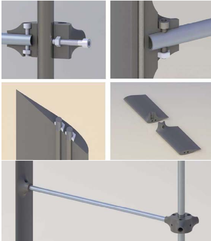
Figure 5.14: New design of the prototype: blades and struts
