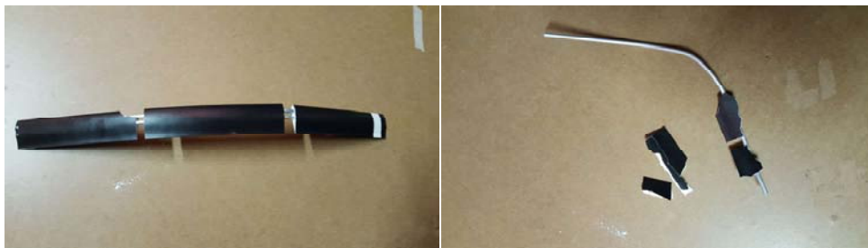
Figure 5.9: Blade failure after testing the first prototype
