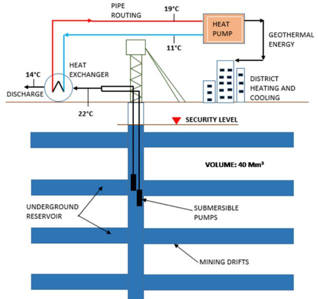
Fig. 3. Geothermal energy production (heating)
