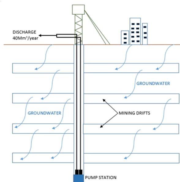
**Fig. 1.** Groundwater and pump system in production phase.
