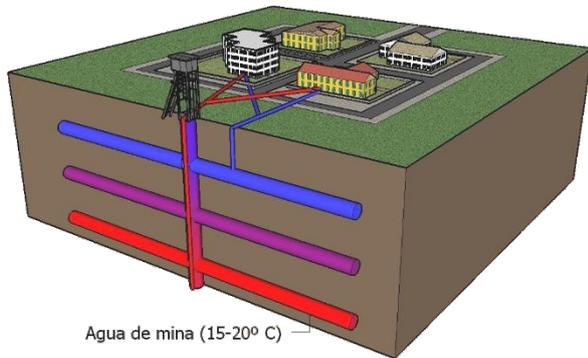
Fig. 2. Geothermal project scheme with mine water
