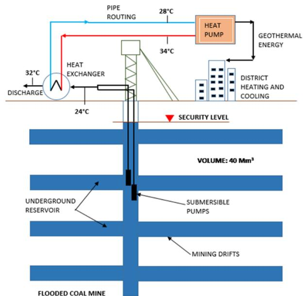
Fig. 4. Geothermal energy production (cooling)
