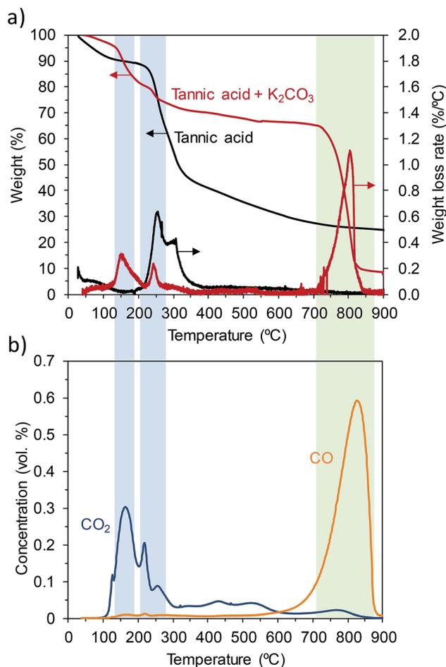
Fig. 3 (a) Thermogravimetric (TGA) and differential thermogravimetric (DTG) curves of the pyrolysis of tannic acid and a mixture of tannic acid and  $\text{K}_2\text{CO}_3$  and (b)  $\text{CO}_2$  and CO TPD spectra obtained from a mixture of tannic acid and  $\text{K}_2\text{CO}_3$  (heating rate:  $3 \text{ }^\circ\text{C min}^{-1}$ ;  $\text{N}_2$  and Ar atmospheres for TGA and TPD experiments, respectively).
