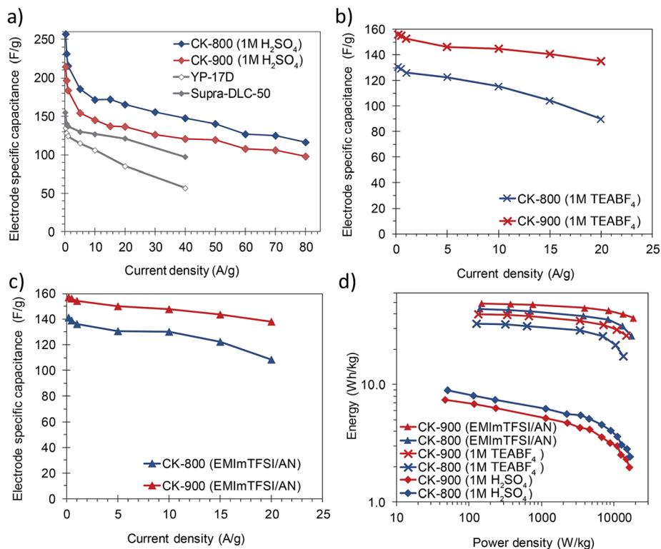
Fig. 5 Rate capability of CK-800 and CK-900 in (a) 1 M H<sub>2</sub>SO<sub>4</sub>, (b) 1 M TEABF<sub>4</sub> and (c) EMImTFSI/AN, calculated by galvanostatic charge-discharge cycling. (d) Ragone plot of the symmetric cells.
