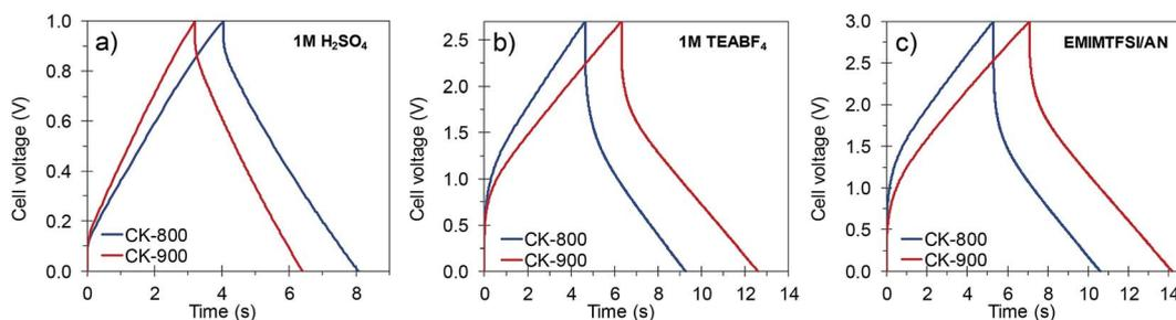
Fig. 6 Galvanostatic charge-discharge profiles of the porous carbons in (a) 1 M H<sub>2</sub>SO<sub>4</sub>, (b) 1 M TEABF<sub>4</sub> and (c) EMImTFSI/AN at a current density of 20 A g<sup>-1</sup>.
