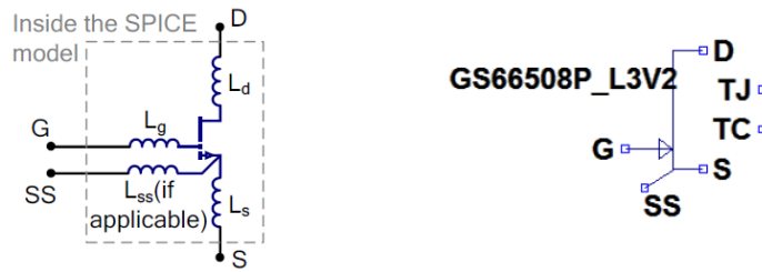
Figure 4-1: Structure and Symbol of the 3-level of GaN systems LTspice model [11]
