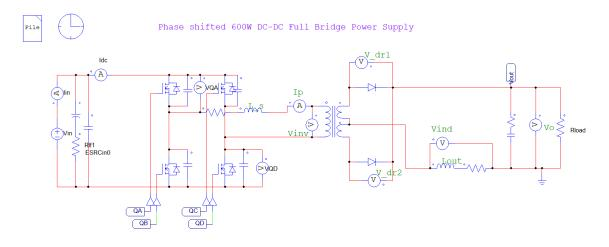
Figure 4-1: Simulation-1: Power stage
