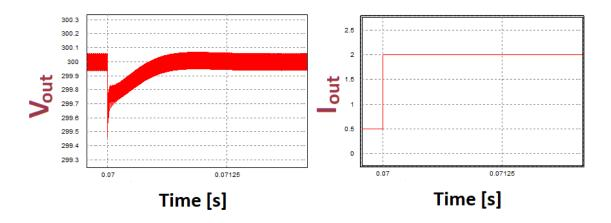
Figure 4-12: 25% to 100% load step response
