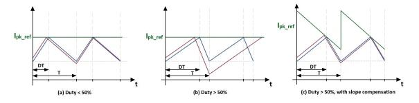
Figure 2-20: Slope compensation on switching inductor current
