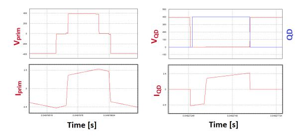
Figure 4-2: Simulation-1: Primary current and voltage, and switching of QD
