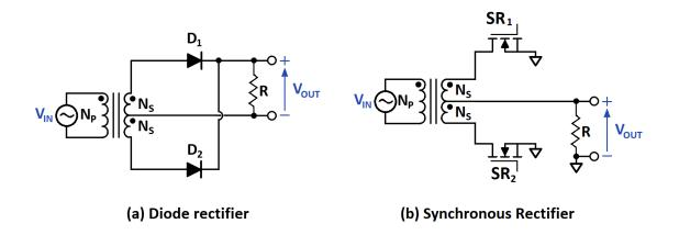
Figure 2-8: Diode rectification vs. Synchronous rectification
