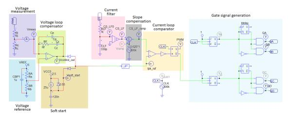
Figure 4-7: Simulation-3: Closed loop control circuit
