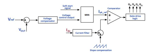
Figure 2-17: Peak current mode control - Control loops
