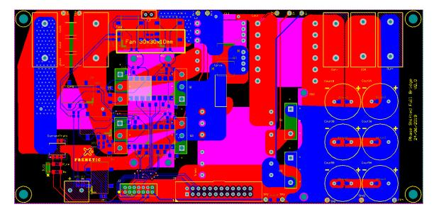
Figure 5-5: Power stage PCB layout on Altium Designer
