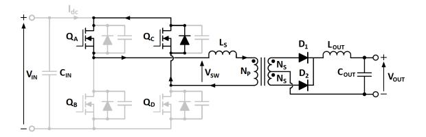
Figure 2-11: Clamped free wheeling interval:  $t_1 < t < t_2$
