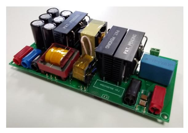
Figure 5-1: Assembled 600W power supply PCB
