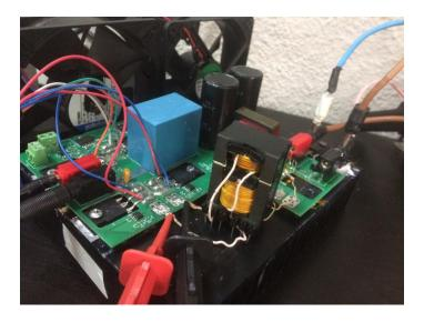
Figure 6-1: Setup of the full power open loop test
