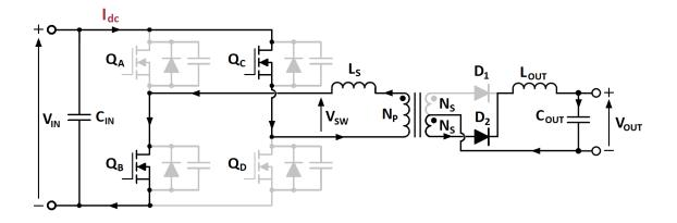
Figure 2-13: Power Transfer Interval:  $t_3 < t < t_4$
