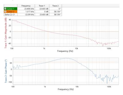
Figure 6-11: Bode analyzer loop stability test results
