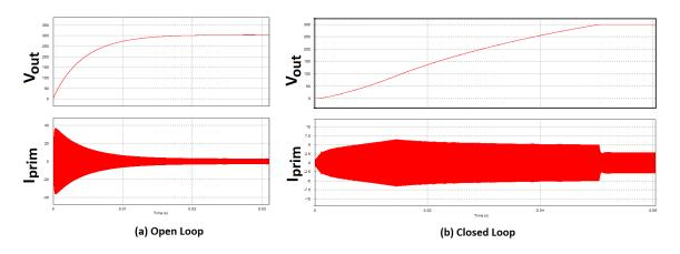
Figure 4-8: Comparison of primary current and voltage transients
