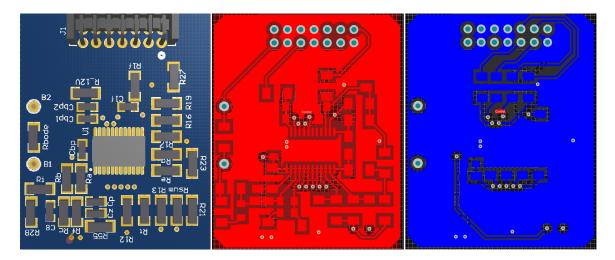
Figure 5-6: Control PCB layout on Altium Designer (3D, top, bottom)
