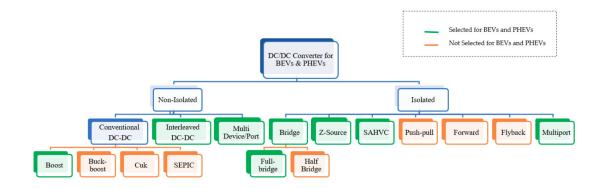
Figure 2-1: Classification of DC-DC converter topologies [1]
