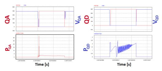
Figure 4-13: Switching transients and instantaneous power losses of leading and lagging leg MOSFETs
