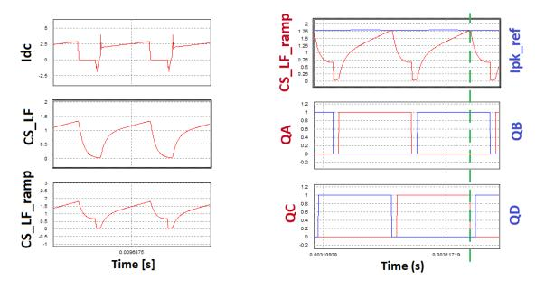
Figure 2-18: Current measurement and ramp compensation
