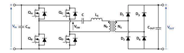
Figure 2-2: Full-bridge LLC resonant converter
