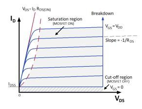
Figure 1-2: Regions of the FET transistor on the IV
