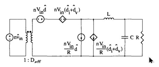
Figure 2-16: Small-signal circuit model of PSFB converter [14]
