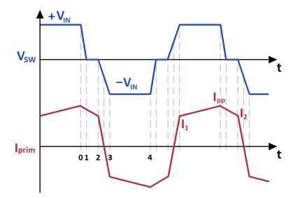
Figure 2-14: Voltage and current wavforms  $t_0 < t < t_4$
