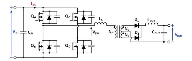
Figure 2-5: Phase-Shifted Full-bridge converter
