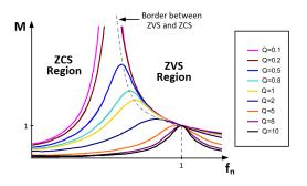
Figure 2-4: Typical gain vs. frequency plot of FB-LLC
