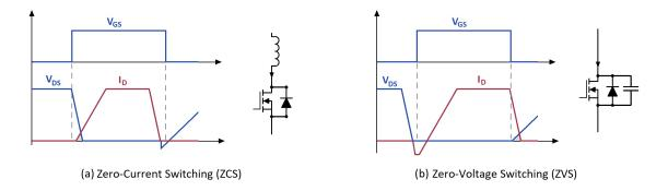
Figure 1-4: Soft switching circuit transients
