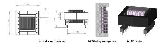
Figure 5-10: Output filter inductor implementation
