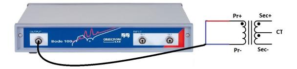
Figure 5-8: Measuring impedance using Bode 100
