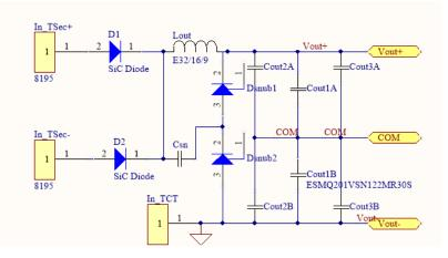
Figure 6-3: Secondary side snubber circuit
