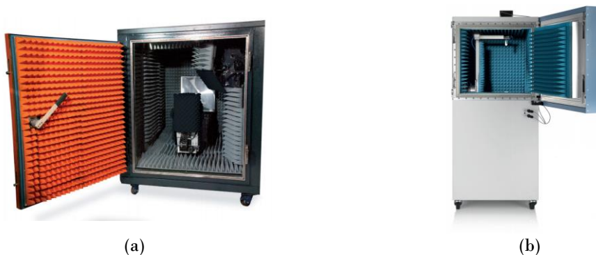
Fig. 3.3. - 5G Measurements products with CATR systems: (a) MVG© Mini Compact Range [21]; (b) R&S©ATS1000 Antenna Test System [22].
