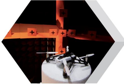
Fig. 2.5. - Over-The-Air (OTA) drone measurement [10].
