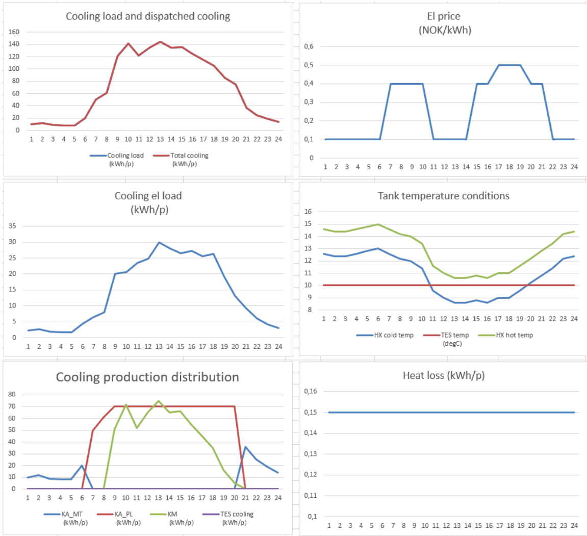
Figure 4-17: Base case in summer operation - the energy exchange variable is fixed to zero
