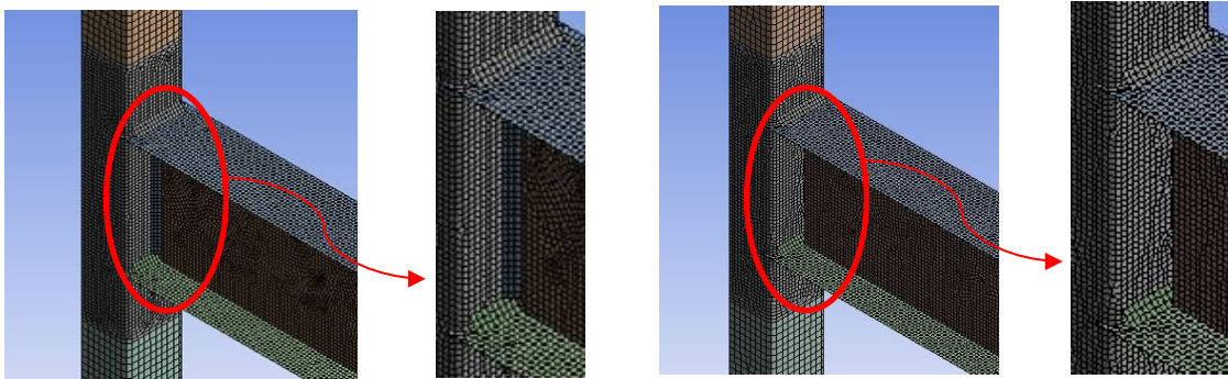
Fig. 9. Finite Element meshes for F+W (left) and F (right)
