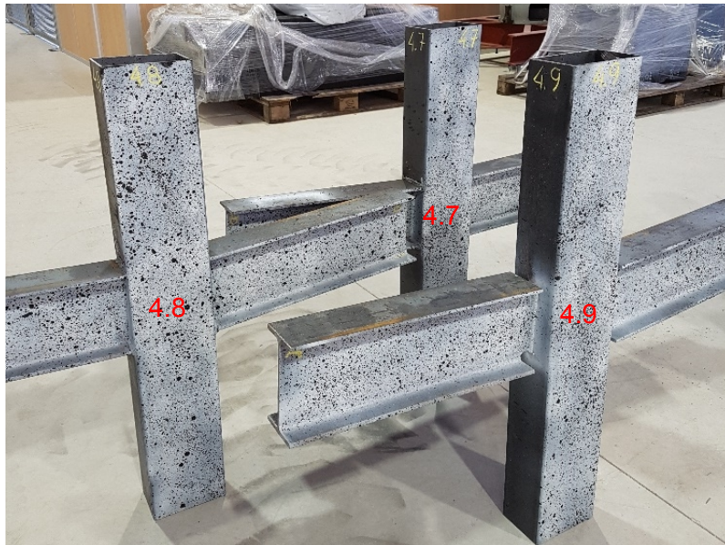
Fig. 1. One set of specimens: 4.7 with all the perimeter welded (F+W), 4.8 with only the flanges welded (F) and 4.9 with only the web welded
