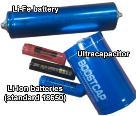
Fig. 1: Set of batteries and ultracapacitors
