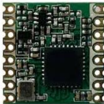
Figura 18 Transceptor LoRa RFM95W
