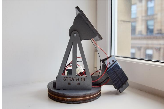
Figure 30: Concept 2 full structure facing the direction of maximal power output for the horizontal axis
