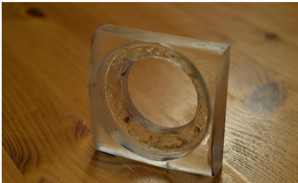
Figure 68: Failed Connection Piece Housing
