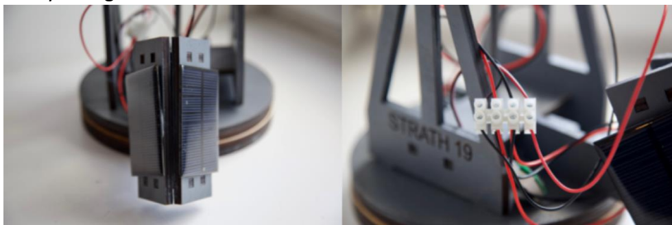
Figure 29: Oppositely facing solar panels (left) wiring connecting panels to motor in reverse polarity (right)
