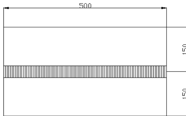
Fig. 5.7 Dimensions of welded plate
