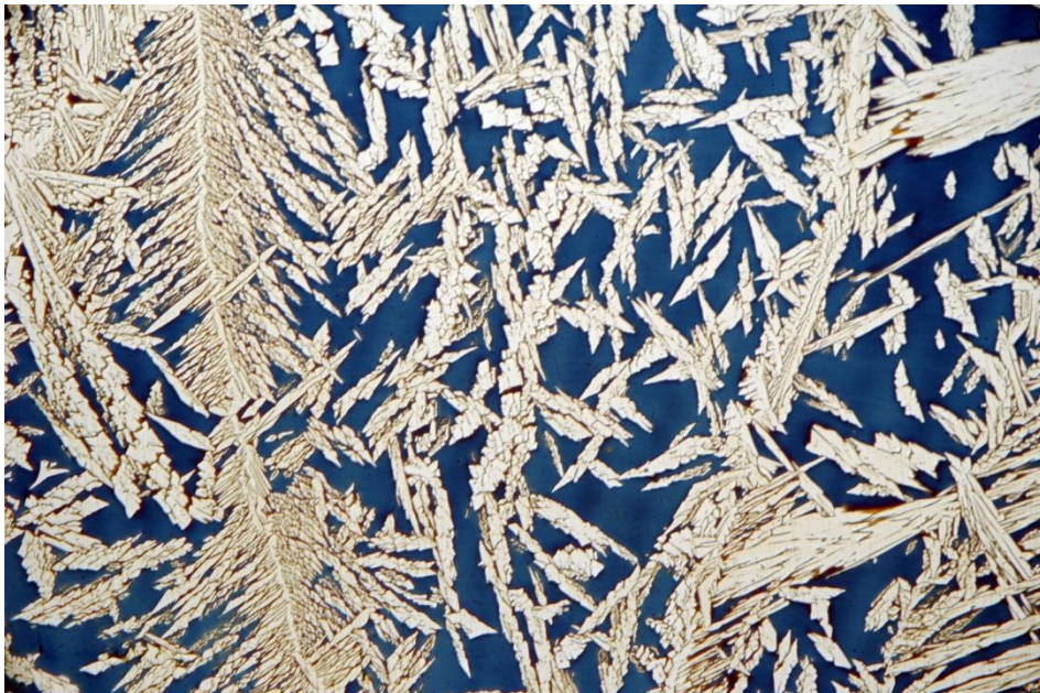
Fig. 5.15. The structure of weld metal (point 4). 2205 duplex stainless steel welded joint. Magn. a) 100 x, b) 250 x
