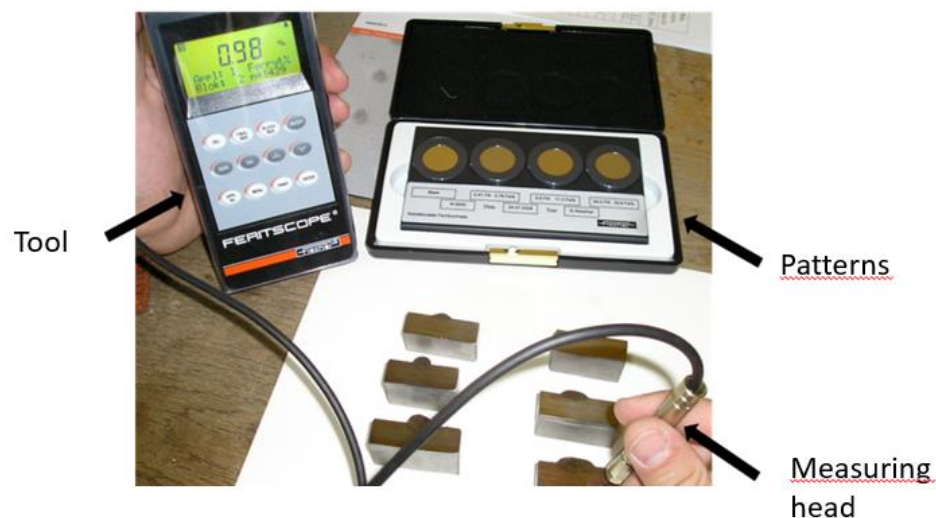
Fig. 5.19 .Ferritometer manufactured by Fisher MP30 company
