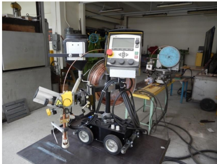
Fig.5.5. ESAB SAW unit used for welding test joint
