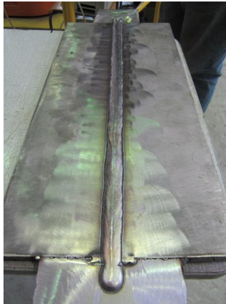
Fig. 5.8. General view of welded plate
