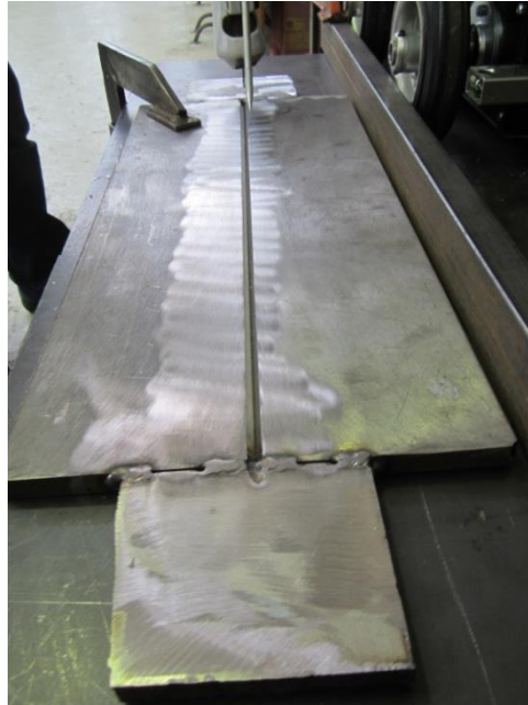
Fig. 5.3. Steel plates before being welded with extra material
