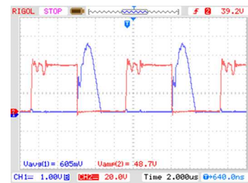
Fig. 17. Switching waveforms of Q_1 : Red: drain-source voltage 20V/div and (Blue) drain current 1A/div.
