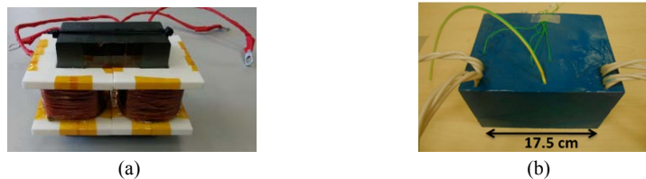
Fig. 5: (a) Non-encapsulated HFT laboratory prototype using two 3-D printed bobbins with 35 turns on each (b) Factory encapsulated HFT. Both designed for a rated power of 5 kW @ 30 kHz with separate windings.
