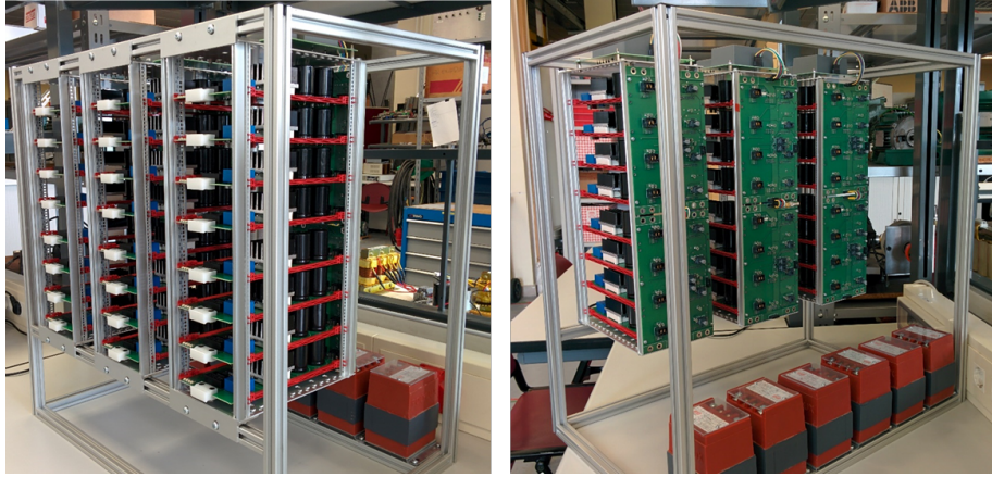
Figure A.5: Eight cells, three-phase MMC prototype. Cells (left) and backplane (right)
