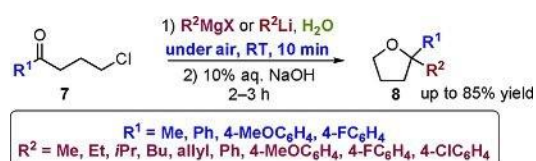
Scheme 4. Addition reaction of organometallic reagents to g -chloroketones 7 "on water", under air and at room temperature, to afford THF derivatives 8.
