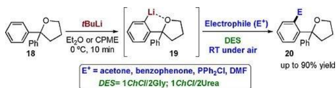
Scheme 9. Ortho -lithiation of diphenyltetrahydrofuran 18 and concomitant functionalisation with different electrophiles in protic eutectic mixtures.
