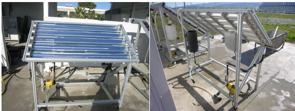
Figure 2.4 – Pilot plant scale CPC solar photoreactor located at the Almeria Solar Platform (Spain).
