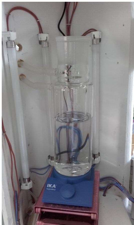
Figure 2.2 – UV-lamps equipped photocatalytic reactor for alkylphenoethoxylates and HMF photo-conversion.
