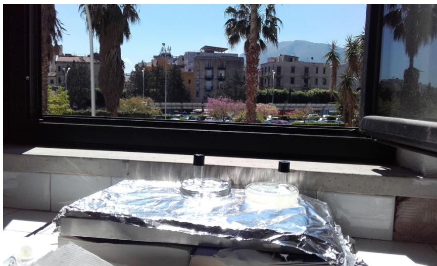
Figure 2.3 – Photocatalytic setup for the natural solar light promoted oxidation of HMF.
