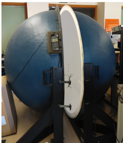
Fig. 4.20. Integrating sphere and spectrophotometer from LabSphere Inc. used for the luminous efficacy and CCT measurements.
