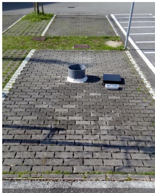
Figure 5. Setup of the infiltration ring for the ASTM C1781/C1781M-15 test on the ICBP surfaces.
