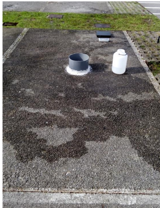
Figure 4. Preparation of the infiltration ring for the ASTM C1701/C1701M-09 test on PMPC and PA surfaces.
