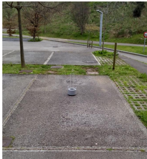
Figure 3. LCS Permeameter ready to begin the NLT-327/00 test on porous-mixture surfaces.
