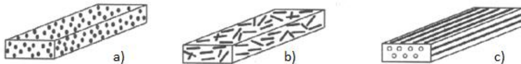
Figure 7.1.- Composite materials with different discontinuous phases: (a) particles, (b) chopped fibers and (c) continuous fibres.
