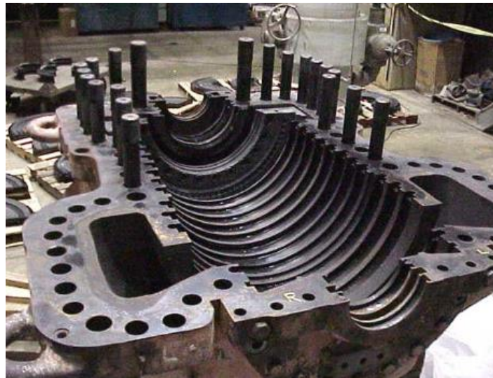
Figure 10. Steam turbine case.
