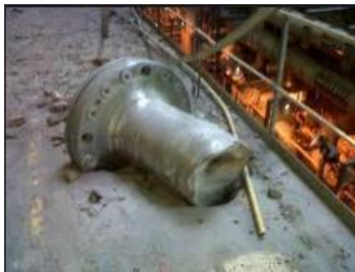
Figure 16. Fragile fracture example.
