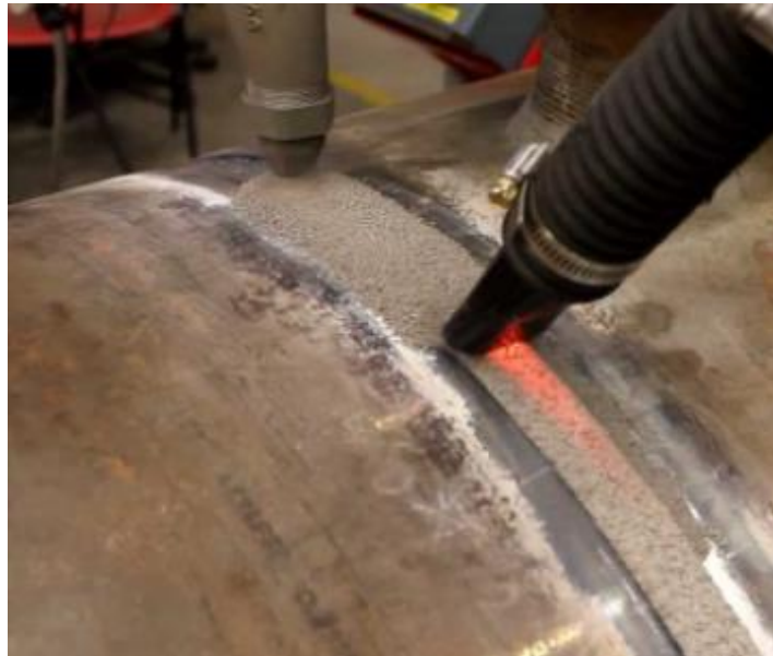
Figure 24. Real submerged arc welding.
