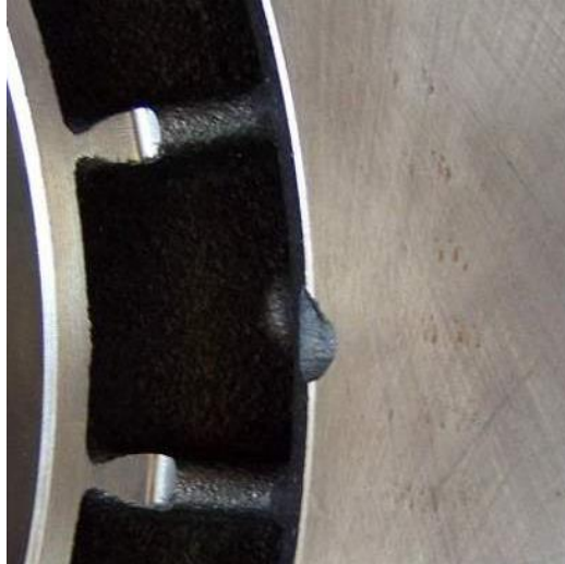
Figure 15. Damage caused by foreign objects.
