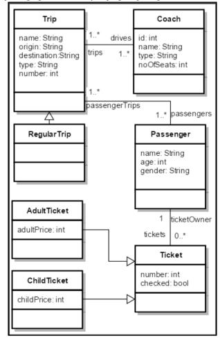
Figure 2 Class diagram for the CDM. It would be desirable to be able to verify on the client as many constraints from Figure1 as possible. The designer must analyze carefully all existing constraints and verify when this is possible.
