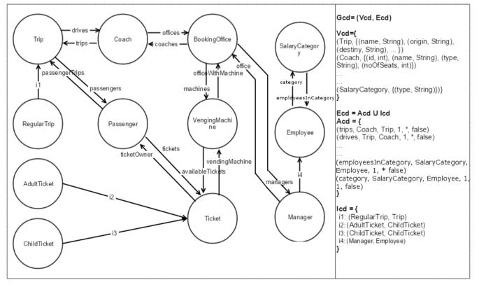
Figure 3: Formal description of the class diagram depicted in Figure 1. It includes a  $V_{cd}$  node set, an edge set that is the union of the  $A_{cd}$  associations sets and the  $I_{cd}$  inheritance relationships set. Only some elements of the sets are shown.
