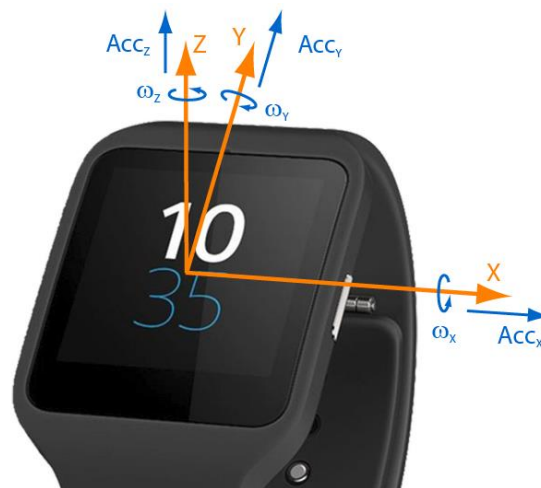
Figure 1: System of reference of the SW3.
