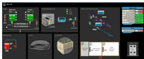
Figura 15: SCADA servicios. Principal
