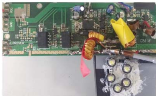
Figure 14. Prototype of the implemented two-phase buck converter with a fourth-order output filter and five LEDs.
