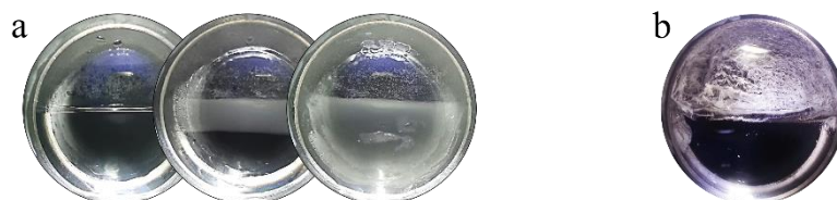
Figure 4. Pictures showing the liquid-gas interphase through the sapphire window. (a) Progress of a turbid front in the liquid phase at the turbidity time. (b) Clathrate hydrate layer over liquid-gas interphase.
