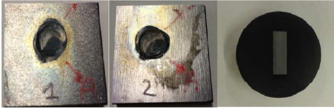
Figure 20. Surface 1 shot peened at 0.4 mmA, surface 2 shot peened at 0.1 mmA and sample of cross section.
