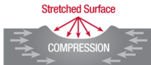
Figure 8. Stresses in a shot peened surface. (Wheelabrator shaping industry)
