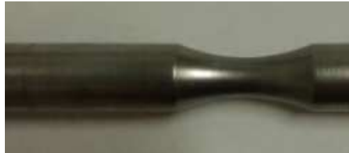
Figure 17. Shot peened sample.
