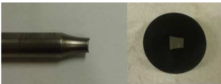
Figure 22. Broken specimen and transversal section sample.
