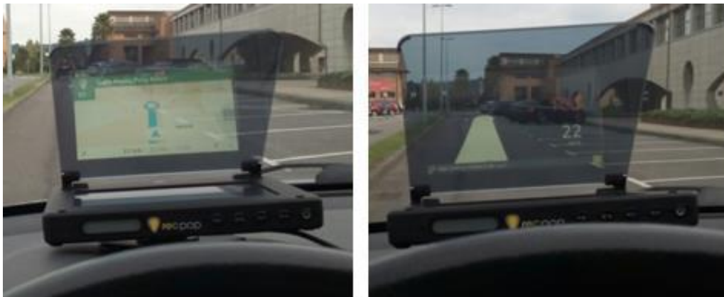
Figure 7. Google Maps (left) and HUDWAY (right) applications running in the HUD device
