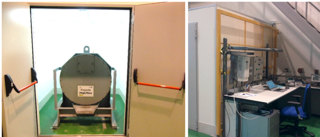
Fig. 7. Test rig overview. Left: Ball mill inside its soundproof room. Right: Control and measurement post next to the soundproof room.
