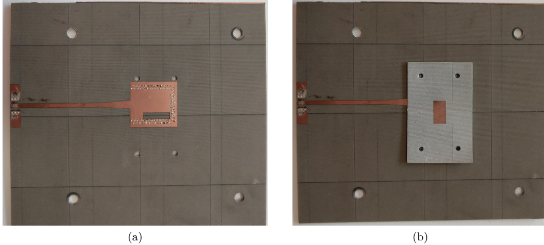
Figure 4.5: Picture of SIW patch antenna with longitudinal coupling slot. (a) Without patch. (b) With patch.
