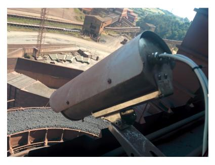
Figure 13. Infrared camera for sinter monitoring.
