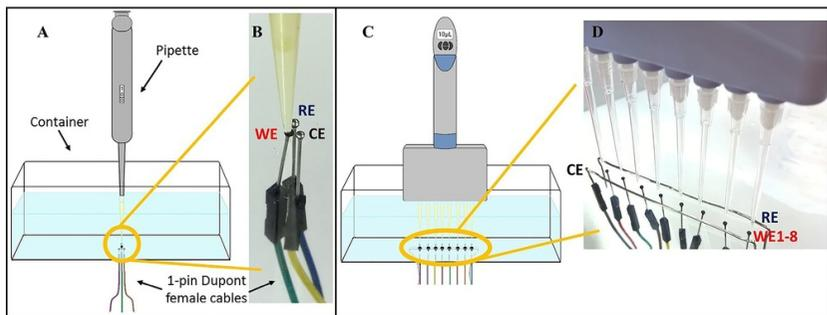
**Fig. 1** (A) Scheme and (B) photograph of amplified detail of the electrode configuration of the single pin-based BIA system. (C) Scheme and (D) photograph of amplified detail of the electrode configuration of the multiplexed pin-based BIA system with eight WEs.
