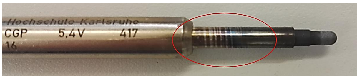
Figure 30. Marks on the CGP after operation in the Adapter
