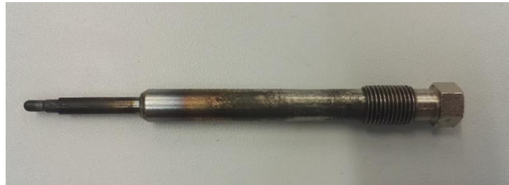
Figure 9. Ceramic part of a CGP located at the inside of this shell [9]
