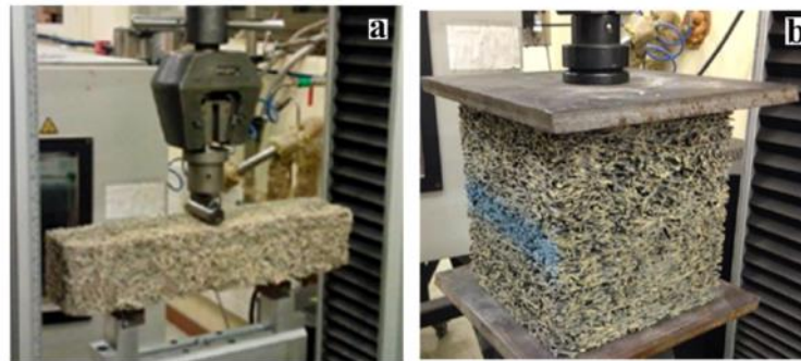
Fig. 1. (a) Bending test; (b) Compression test
