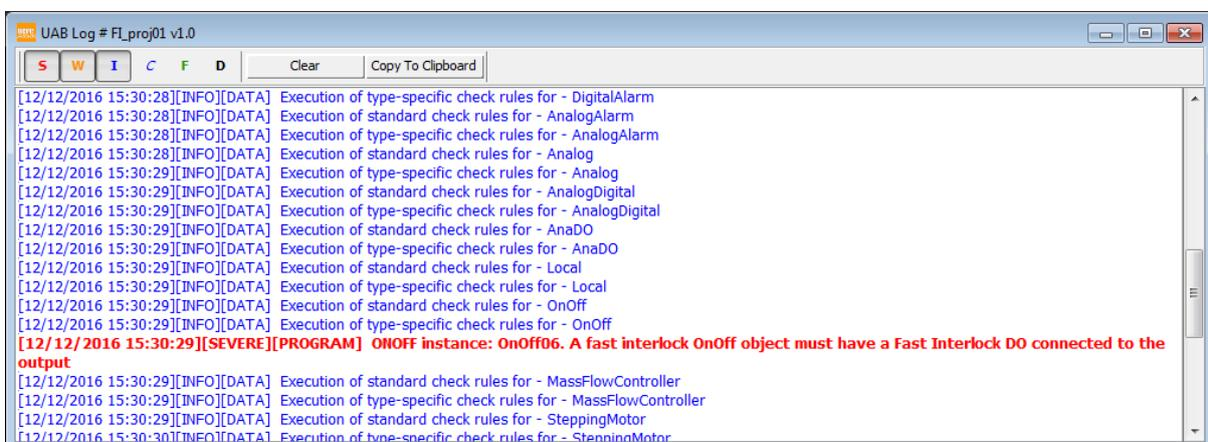
Fig. 11. Normal Digital Output connected to a fast interlock OnOff
