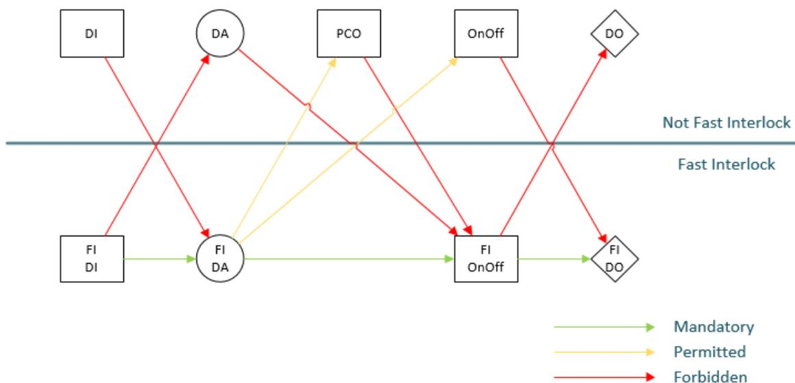
Fig. 7. Interaction between not fast interlock and fast interlock UNICOS objects. Fast interlock objects are placed in the bottom part of the figure
