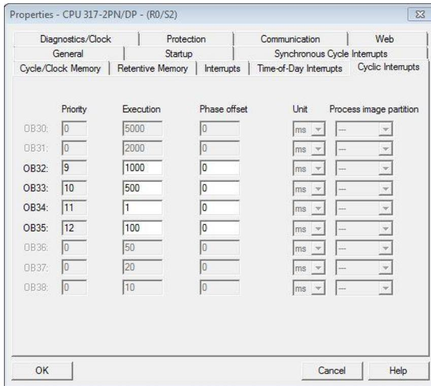
Fig. 9. CPU configuration for cyclic interrupt OB 34
