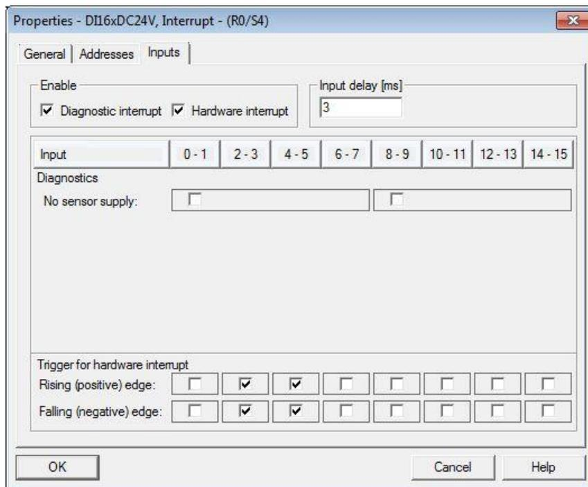
Fig. 8. Digital Input module configuration for hardware interrupts
