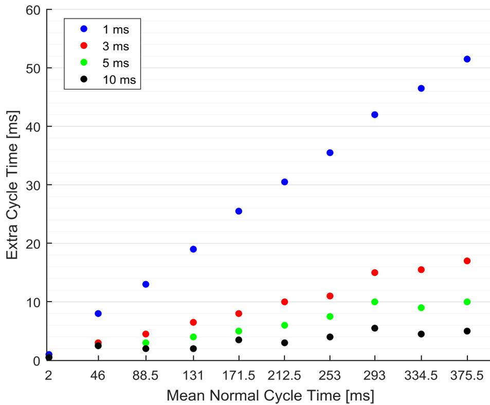
Fig. 3. Extra time for a 1 byte cyclic interrupt input
