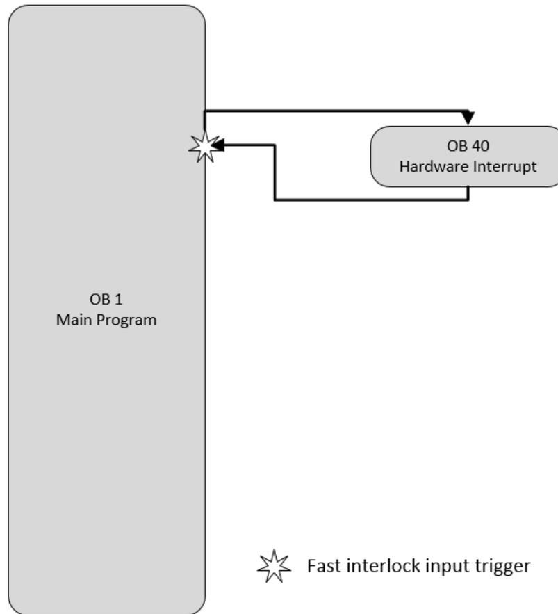
Fig. 1. Hardware Interrupt execution
