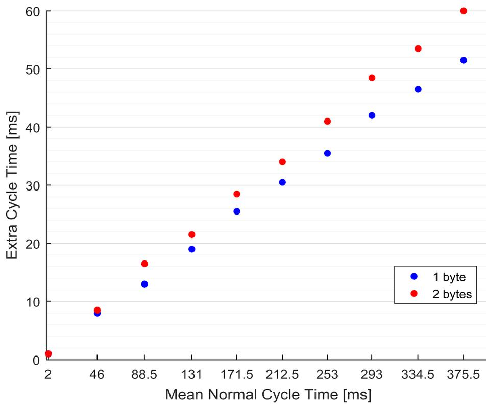
Fig. 2. Extra time for a 1 ms cyclic interrupt
