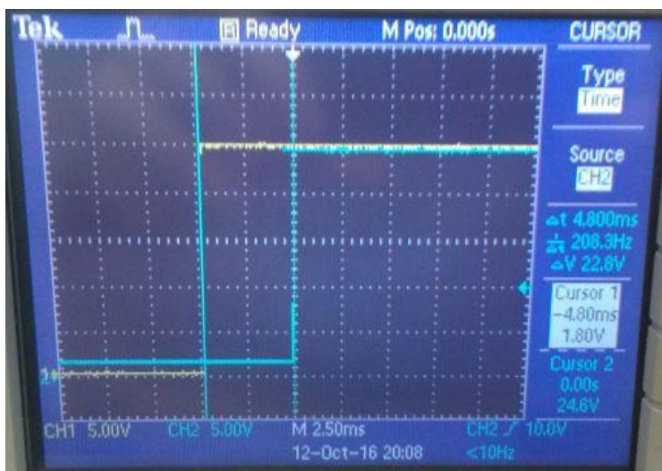
Fig. 20. Oscilloscope cursors used for measurement
