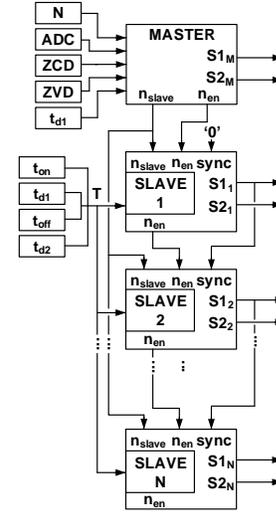
Fig. 8. Master-slave with phase-shedding control diagram.
