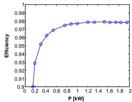
Fig. 13. Measured efficiency of module-type I
