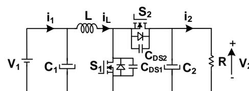
Fig. 1. Synchronous boost converter.
