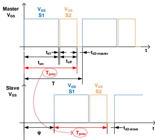
Fig. 3. Example of control waveforms for master-slave solution.
