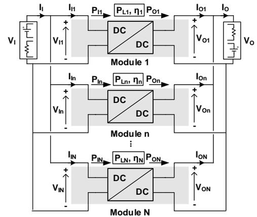
Fig. 6. General IPOP converter composed by  $N$  modules.
