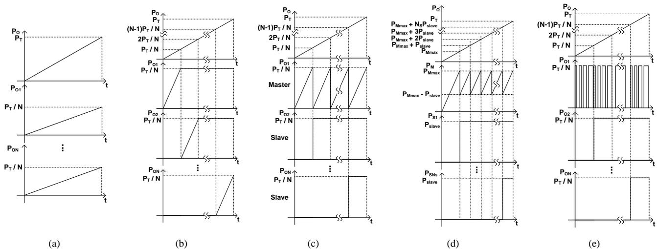
Fig. 7. Power profile example of an IPOP modular converter under different control techniques. (a) Balanced technique. (b) Phase-shedding technique (previous proposed approach). (c) Phase-shedding technique (master-slave approach). (d) Asymmetrical master-slave technique. (e) Burst mode technique.
