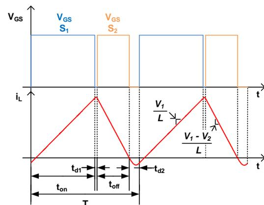
Fig. 2. Theoretical waveforms for a synchronous boost converter operating in QSW-ZVS mode.
