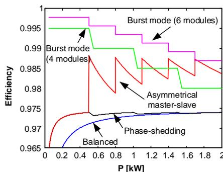
Fig. 10. Overall estimated efficiency comparison of the IPOP modular converter under balanced control, master-slave with phase-shedding, asymmetrical master-slave and burst mode (with 4 and 6 modules).
