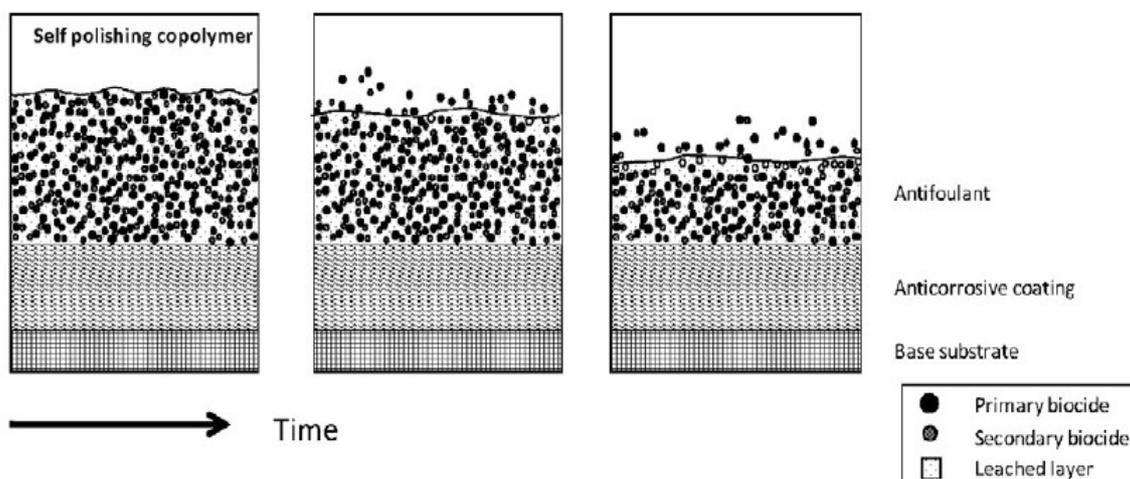
Fig.2 Self-polishing copolymer [3]
