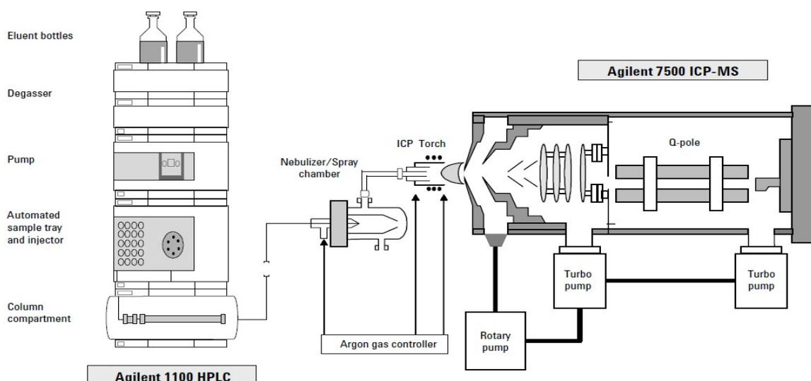
Fig 20. Schematic of the HPLC-ICPMS instrumentation
