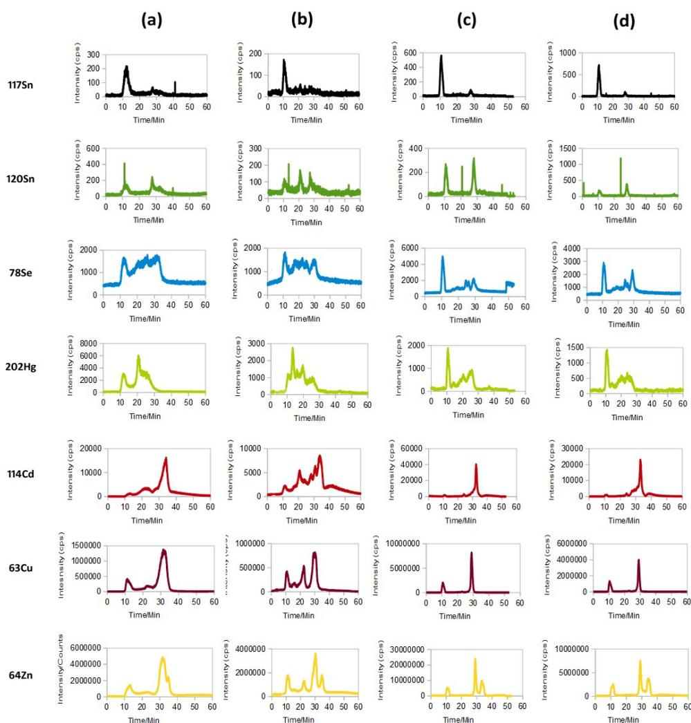
Fig. 27. Tin, cadmium, copper, zinc, selenium and mercury chromatograms. (a) Digestive tract,  $^{117}\text{TBT}$  dissolved in phytoplankton, (b) Digestive tract,  $^{117}\text{TBT}$  dissolved in water, (c) Gills,  $^{117}\text{TBT}$  dissolved in water, (d) Gills,  $^{117}\text{TBT}$  dissolved in phytoplankton
