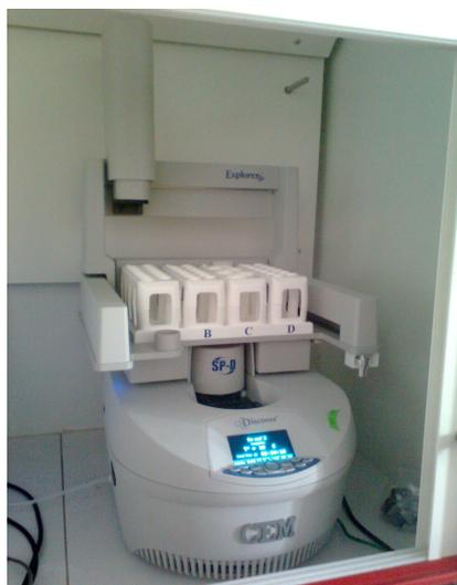
Fig. 15. Analytical MW Digestion system used at the IPREM
