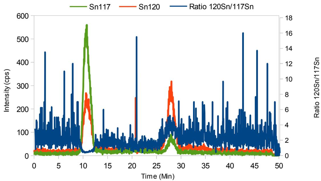
$^{120}\text{Sn}$  and  $^{117}\text{Sn}$  chromatograms vs  $^{120}\text{Sn}/^{117}\text{Sn}$  for gills with  $^{117}\text{TBT}$  phytoplankton enrichment
