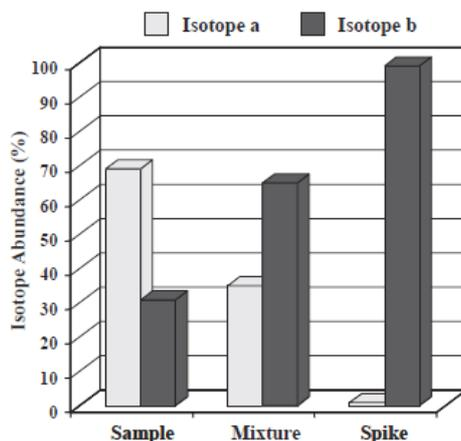
Fig 3. Illustration of the principle of isotope dilution analysis for an element combining two different isotopes A and B [11]
