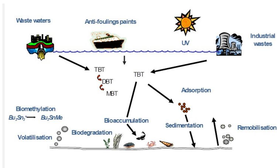
Fig.3 Sources and fates of TBT into biodegradation, bioaccumulation and storage in aquatic systems
