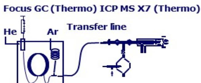
Fig 18. Scheme of the GC-ICP MS instrumentation
