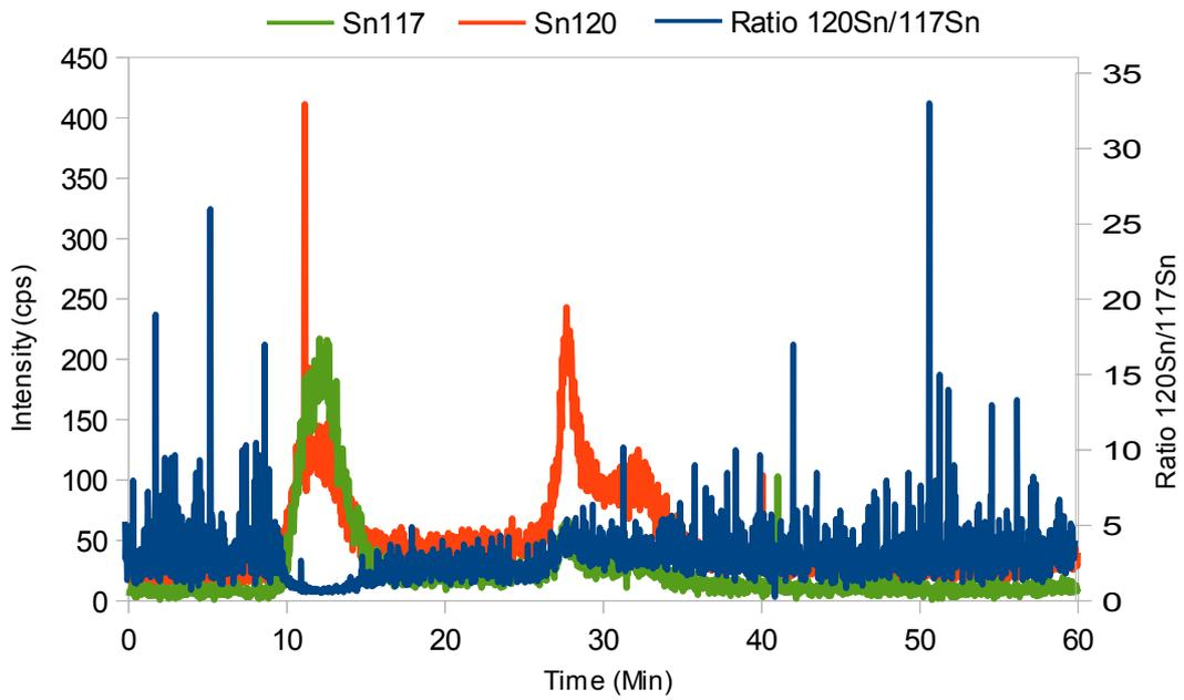
$^{120}\text{Sn}$  and  $^{117}\text{Sn}$  chromatograms vs  $^{120}\text{Sn}/^{117}\text{Sn}$  for digestive gland with  $^{117}\text{TBT}$  phytoplankton enrichment
