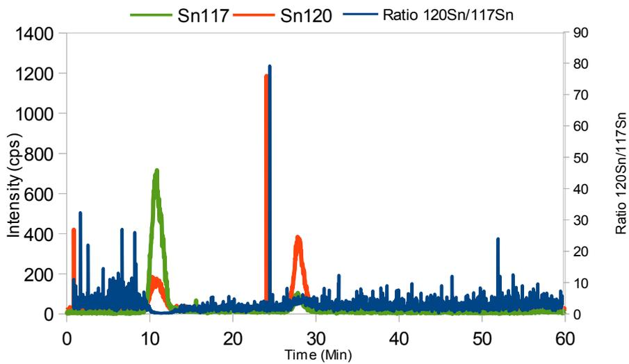
$^{120}\text{Sn}$  and  $^{117}\text{Sn}$  chromatograms vs  $^{120}\text{Sn}/^{117}\text{Sn}$  in the case of gills with  $^{117}\text{TBT}$  water addition
