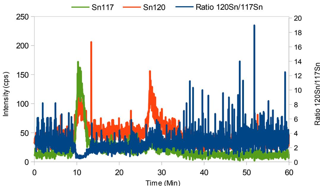
Fig. 29.  $^{120}\text{Sn}$  and  $^{117}\text{Sn}$  chromatograms vs  $^{120}\text{Sn}/^{117}\text{Sn}$  for digestive gland with  $^{117}\text{TBT}$  water addition
