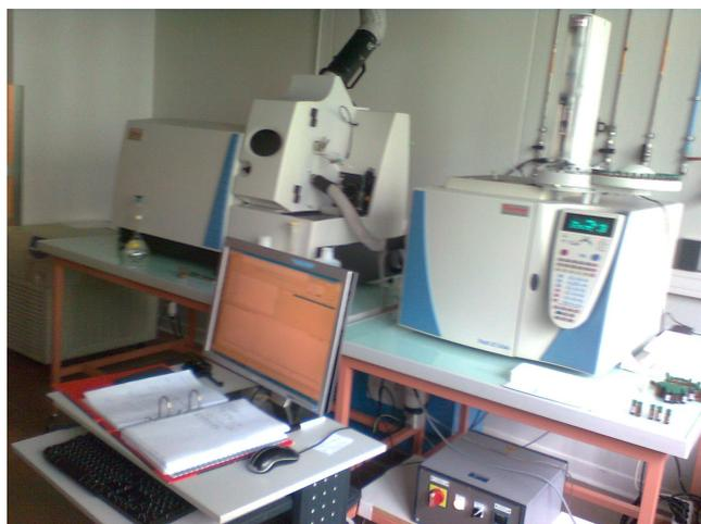
Fig. 19. GC-ICP MS used at the IPREM
