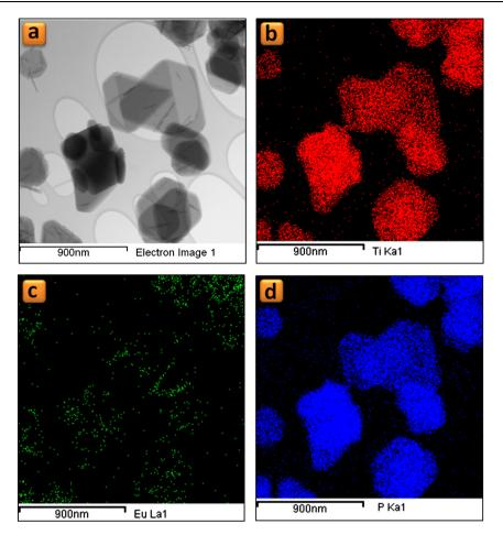
Figure 4 Elemental mapping for TiP\_0.1 sample: (a) Bright field-STEM images, (b) Ti-K $\alpha_1$  map, (c) Eu-L $\alpha_1$  map and (d) P-K $\alpha_1$  map.
