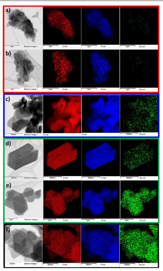
Figure 9 STEM-EDS elemental mapping of TiPPr\_x samples ( $\mathbf{x} = 10^{-4}$  (a),  $10^{-3}$  (b), 0.05 (c), 0.075 (d and e) and 0.1 (f)); Ti-K $\alpha_1$  (red), P-K $\alpha_1$  (blue) and Eu-L $\alpha_1$  (green) elemental maps.
