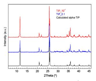
Figure 1 PXRD patterns of the samples  $TiP_10^{-4}$  (red) and  $TiP_0.1$  (blue), and calculated for  $\alpha$ -TiP (black).
