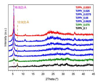
Figure 6 PXRD patterns of the TiPPr\_x samples.
