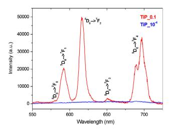
Figure 5 Emission spectra of the samples  $TiP_0.1$  (red) and  $TiP_10^{-4}$  (blue) obtained up excitation at 394 nm.
