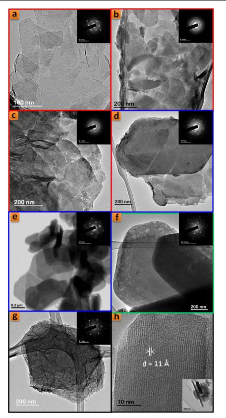
Figure 8 TEM images of TiPPr\_x samples (x =  $10^{-4}$  (a),  $10^{-3}$  (b), 0.01 (c), 0.025 (d), 0.05 (e), 0.075 (f) and 0.1 (g and h)).
