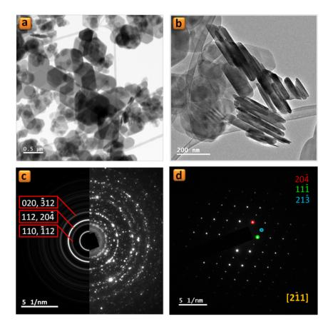
Figure 2 (a and b) TEM images, (c) selected area electron diffraction (SAED) patterns (left: simulated, right: experimental), and (d) nanobeam electron diffraction (NBD) pattern along [2–11] zone axis for a single particle of  $TiP_10^{-4}$  sample.
