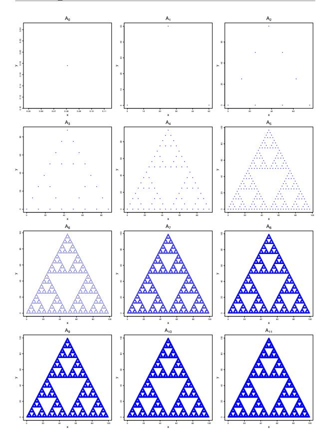
Figure 4.2: Progression of a Sierpinski Triangle in  $\mathbb{R}^2$  by Implementing the Deterministic Algorithm
