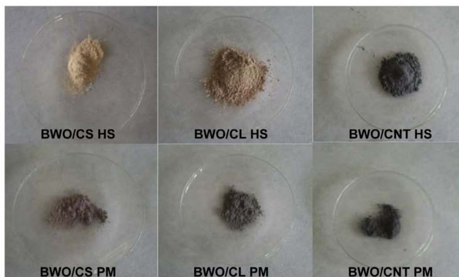
Fig. 1. Images of hybrid catalysts prepared by incorporation of the carbon additive before the hydrothermal synthesis of the semiconductor (series HS) or by physical mixture of the carbon and \text{Bi}_2\text{WO}_6 powders (series PM).
